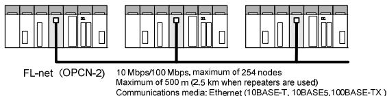
FL-net (OPCN-2) is an open, multi-vendor network, which not only allows high-speed data transfer between FA-M3 units but also connection to third-party FA controllers.
