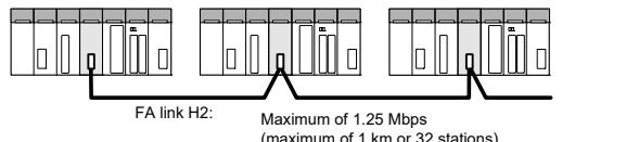
Use the FA link H2 modules for exchanging data between FA-M3s.
