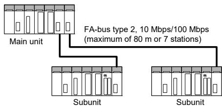
Use a FA-bus Type 2 module when adding subunits.
