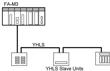
YHLS (Yokogawa Hi-speed Link System) enables easy implementation of high-speed 1:N remote I/O communication systems.
