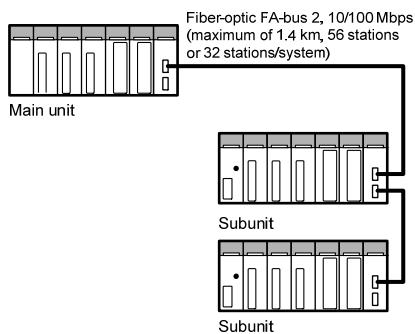
Use a fiber-optic FA-bus Type 2 module when augmenting I/O devices in a multi-station or long distance configuration.
