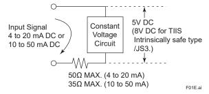
Figure 1. Equivalent Circuit
